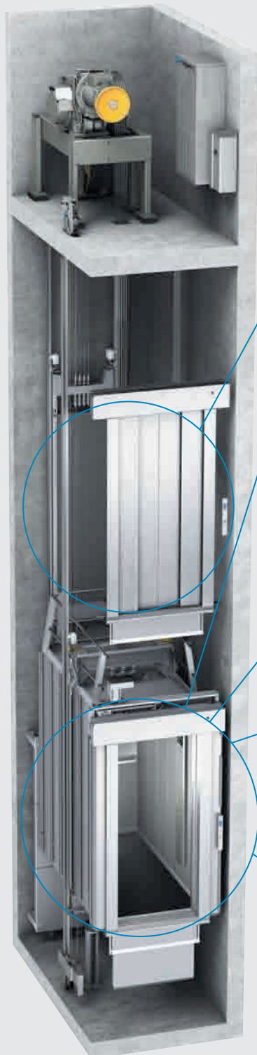
Pictured: - with geared drive in the machine room
